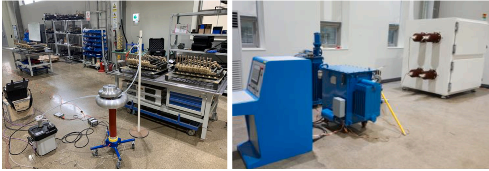
Fig. 2. Overview of the ALT setup. Left: diagnostic configuration for partial discharge, dielectric loss tangent ( \tan \delta ), and insulation resistance measurements; Right: high-temperature and high-voltage endurance chamber and transformer-based power supply system.
