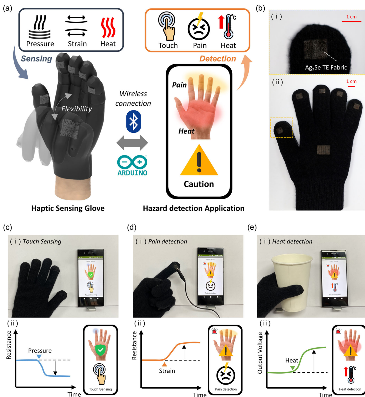
Figure 4. a) Schematic illustration of the haptic sensing glove-based potential hazard detection system. b) Optical image of the haptic sensing glove. c) (i) Demonstration of touch sensing using the haptic sensing glove. (ii) Pressure sensing-based touch sensing mechanism. d) (i) Demonstration of pain detection using the haptic sensing glove. (ii) Strain sensing-based pain detection mechanism. e) (i) Demonstration of heat detection using the haptic sensing glove. (ii) Output voltage sensing-based heat detection mechanism.
