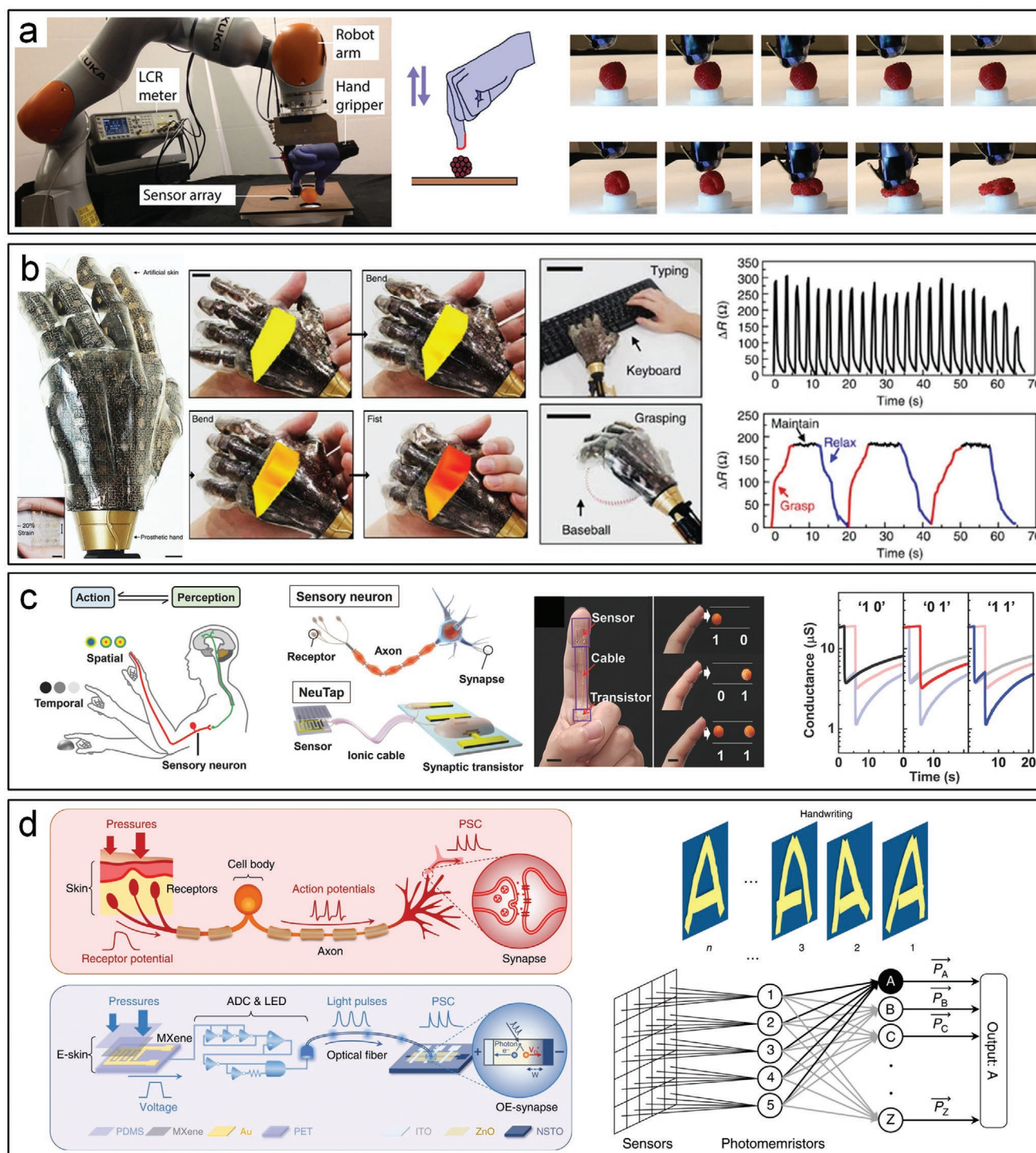
Figure 11. Artificial electronic skins for robotic and prosthetic applications. a) Robotic gripper equipped with closed-loop tactile feedback capable of interacting with fragile objects. Reproduced with permission. [165] Copyright 2018, AAAS. b) Artificial skin for a prosthetic limb that responds to daily life situations. Reproduced with permission. [169] Copyright 2014, Springer Nature. c) Artificial sensory neuron that mimics human perceptual learning. Reproduced with permission. [172] Copyright 2018, Wiley-VCH. d) Bioinspired, artificial optoelectronic afferent nerve systems that can recognize and learn handwritten words. Reproduced with permission. [175] Copyright 2020, Springer Nature.
