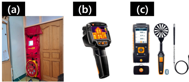
Fig. 5. Instruments for measuring airtightness: (a) blower door test, (b) Testo 872, (c) Testo 440.
